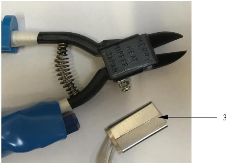
4. Insert the new heating element, make sure it has good contact with the gate cutters surface, tighten the Philips screw, and reconnect the plug.
